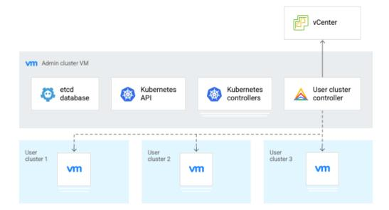
The following diagram shows a more complete example of GKE on VMware deployed in a hybrid environment. Additional services like Config Sync, Binary Authorization, and Operations Suite supplement the on-premises GKE services that run in VMware:
