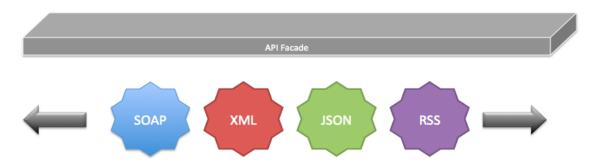
With a facade pattern in place, apps that consume the external services can expect a canonical model to consume the APIs. Also, if implemented through the facade, the external services can easily be plugged and replaced.
