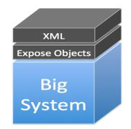
In the build-up approach, a developer exposes the core objects of a big system and puts an XML parsing layer on top.
