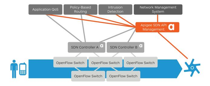
Figure 1 Connecting the SDN ecosystem and optimizing end-user experience.
