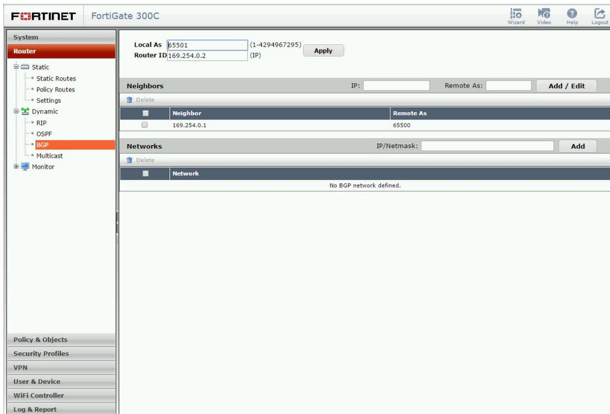
The screenshot displays the Fortinet FortiGate 300C configuration page for BGP. The left sidebar shows the navigation menu with 'Router' expanded and 'BGP' selected under the 'Dynamic' section. The main configuration area is divided into sections for 'Local As', 'Neighbors', and 'Networks'.
